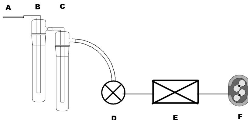
FIG. 1. Diagram of the small-scale smoke machine used during the experiments: A, cigarette; B, solvent trap one; C, solvent trap two; D, suction volume regulator; E, puff frequency and puff duration regulator; F, vacuum pump.
